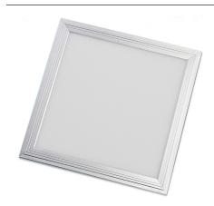
The Thebe Ultra Slim LED panels are thin, optical acrylic sheets with high output tier one LEDs embedded along the edge of the LED Light Panels and an engraved light distribution matrix across the back of the panel.
